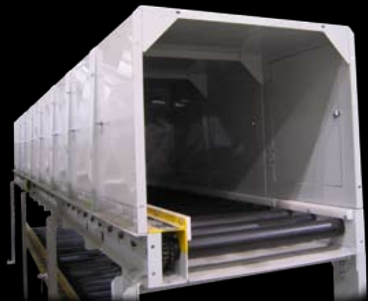
Conveyor equipped with hood to capture effluent gases released during core cooling process
