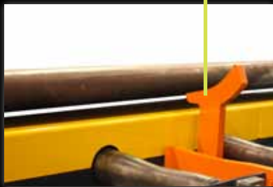
■ Concave rollers for tube cradling
