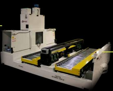
Heavy rollers with flange mounted bearings at end to withstand impact loading
