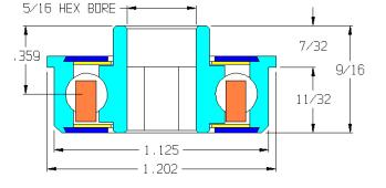
Recommended for medium to heavy loads in dirty environments. Metal shields deflect large particle debris and protect sealing rings that block smaller dirt and debris. Not effective against small particle dust. Light oil offers very little rotational drag making this bearing highly recommended for gravity applications with light products.
