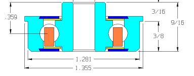
Recommended for medium to heavy loads in dirty environments. Metal shields deflect large particle debris and protect sealing rings that block smaller dirt and debris. Not effective against small particle dust. Light oil offers very little rotational drag making this bearing highly recommended for gravity applications with light products.
