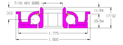
Designed specifically for 2" OD tubing. Light oil offers very little rotational drag making this bearing highly recommended for gravity applications with light products. A polymer sealing ring holds out large particle debris but is not effective against heavy dust and small particles. The light oil is not recommended for powered applications where the bearing is rotating continuously.
