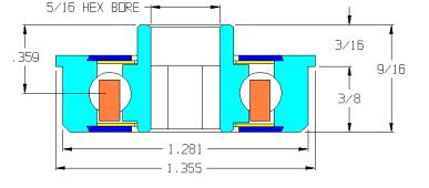
Recommended for medium to heavy loads in dirty environments. Metal shields deflect large particle debris and protect sealing rings that block smaller dirt and debris. Not effective against small particle dust. Grease keeps this bearing lubricated for continuous use but increases the rotational drag. Not recommended for gravity applications with light products.
