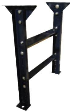
3 1/2" x 7 ga. formed channel mild steel, powder coated bolt-together leg supports
